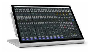
on multiple PC screens from a cloud. Glass LXE can be used alone or combined with the physical LXE surface to give broadcasters full console control anywhere that's needed on a UI that is very familiar.
