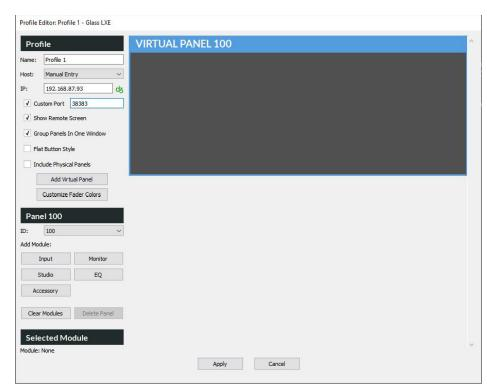
Now it's time to define some Virtual Panels. Virtual Panels host modules. So before we can add any input or output modules we need a panel to host them. Virtual Panel ID's start 100 by default. This is fine, and should be left at default numbering. The Next Panel will have id of 101.
