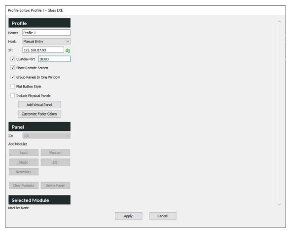
The next option is the Custom Port option. This is the Port for Glass LXE to connect to the surface with. Check Use Custom Port, and enter 38383. This port is designated as the default connection port for Glass LXE connections. This can be changed to suit your network if needed.
