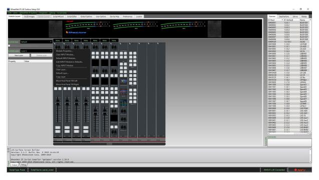
Right click on an Input Module and select Default INPUT Module. This will assign Default Functions to the Controls on the Input Module.
