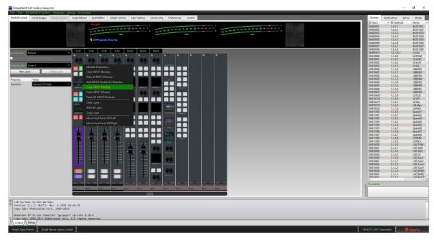
Once the first module has default values, you can right click and copy this module using the Copy function, then right click on the next Fader and select Paste INPUT Module, or do the rest of the input modules with Paste All INPUT Modules.
