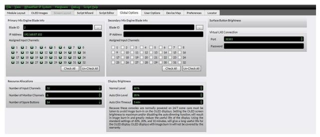
In the Global Options Screen, we need to tell the LXE Surface Host, which Blade on the Network is it's Mix Engine. If you have not already done so, click Wheatnet\_IP\_System and select Scan. Enter a Valid Blade IP address as the Starting point for the Scanner. When the System Scan Finishes, click Use this Scan information. When prompted Save the scan file in the default directory offered.
