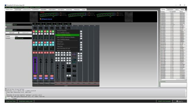
When you select Default Output Module, you will get an extra options window for the type of output module you are configuring, i.e., a CR, or HP Monitor, or a Studio Monitor. Our first Output Module, is typically the CR module.
