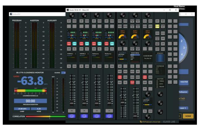
Your Glass LXE Surface is now ready to bring in sources and mix to outputs. You will need to make crosspoints in the Navigator Software to bring Monitor Sources from the Surface to Blade Outputs, wired to speakers or headphones.
