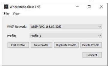
Select the WNIP Network NIC, to bind the application to the WheatNet-IP Network interface on the PC.
