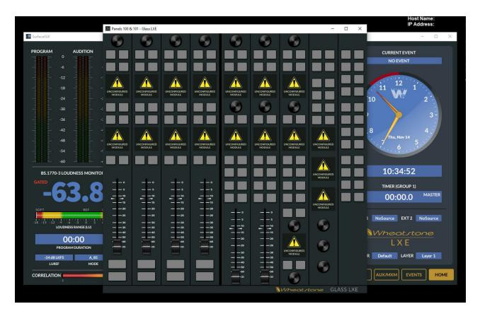
Running Profile 1, notice the modules grouped into 1 window. The surface Screen has it's own window behind the modules displayed. The Triangle with! means that the Modules are not configured yet.
