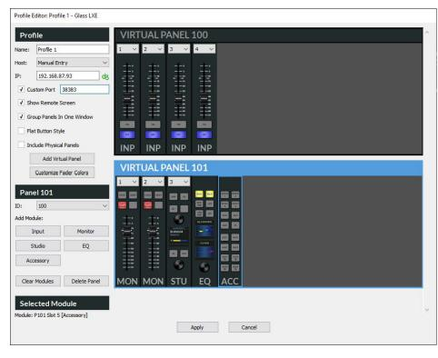
To add modules to a panel, select the Target Panel on the right, then selectthetypeofModule you want to add to each panel. Remember that in our options above, we've selected to group panels into one window. Later when we run this profile, these panels will show up in a single window. If we unchecked that option, when we run the profile, each panel would have it's own window. This is handy in multiple monitor/screen setups if using them.
