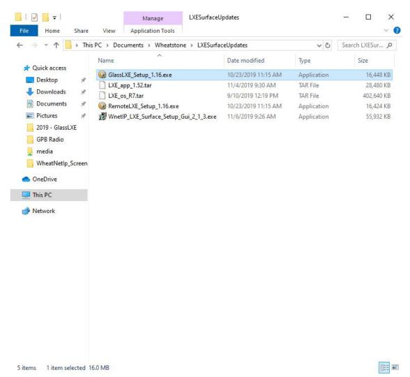
Select the GlassLXE\_Setup\_1.16.exe file and double click it to start the installation wizard.
